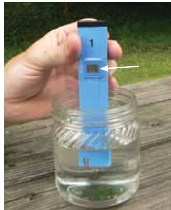
Immerse the bottom of the tester 1 inch to 3.5 inches into water sample. Gently stir the water with the tester for several seconds until the digital display stabilizes. Once display stabilizes, read your TDS value.
